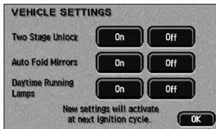
After touching the **Vehicle Settings** button, the screen displays the buttons that switch certain functions on or off.
